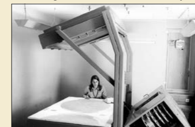
A prototype of BESSY, the scanning table designed specifically for use on film from BEBC, delivered to CERN in December 1971. (Image credit: CERN-EX-7204071.)
