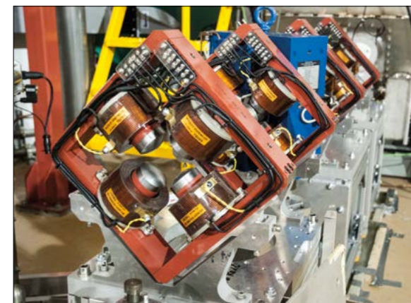
Fig. 3. Close-up of the "short" quadrupoles used in the electron-beam transport line. These TRIUMF-designed magnets employ a novel pole design that presents minimal aberrations to the electron beam.
