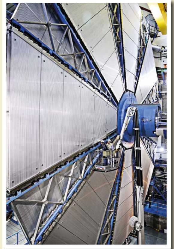
Below right: Members of the ATLAS muon team inspect the monitored drift tubes of the muon spectrometer before the shielding that encircles the beam pipe, where collisions occur, is installed. The shielding is designed to maintain the integrity of the beam and to protect the sensitive components of the detector near the beamline. (Image credit: Claudia Marcelloni.)
