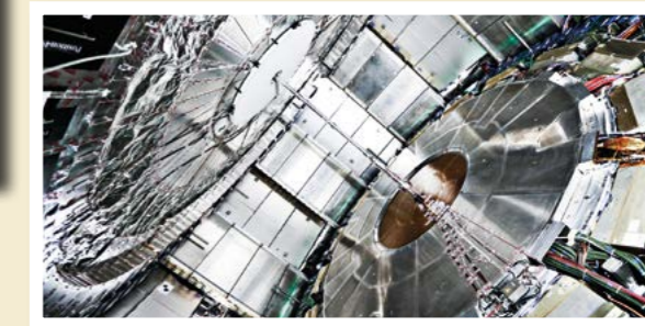
Below: View of the ATLAS calorimeters from below as they were being moved to their final position before the detector closed for the LHC's second run. Calorimeters measure energy carried by neutral and charged particles. (Image credit: Claudia Marcelloni.)
