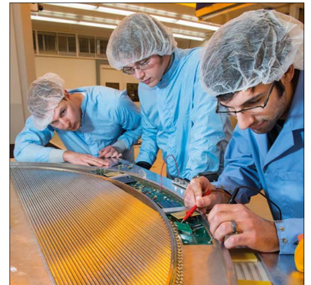
Fig 3. This prototype Mu2e tracker panel consists of 96 straw tubes arranged in two layers. Postdoctoral research associates (left to right) Jason Bono, Dan Ambrose and Richie Bonventre install the read-out electronics. (Image credit: Reidar Hahn/Fermilab.)
