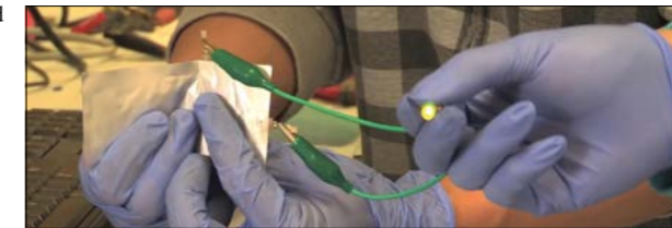
The prototype aluminium-ion battery under test. (Image credit: Stanford University.)
