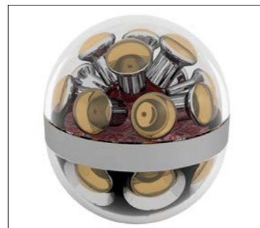
Concept for an IceCube-Gen2 multi-PMT digital optical module (OM), motivated by the OM from KM3NeT. (Image credit: Alexander Kappes.)
