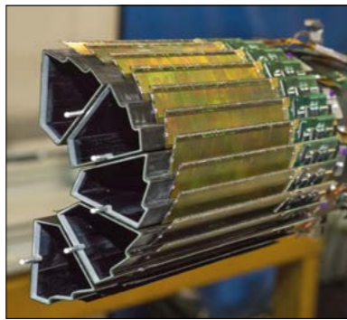
Fig. 1. One half of the PXL detector, showing 50 \mu\text{m} -thick MAPS sensors mounted on their carbon-fibre supports. The complete detector consists of 400 MAPS sensors arranged into two layers at radii of 2.8 and 8 cm from the beamline. The outer layer is visible here. (Image credit: Berkeley Lab/Roy Kaltschmidt.)
