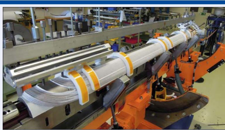
On 16 June, an 11 T superconducting dipole-magnet model manufactured at CERN for the High-Luminosity LHC project reached record performance levels in tests in hall SM18. Its magnetic-field intensity exceeded 11 T after just six quenches – a much faster increase than in previous models. In addition, it reached 12 T – corresponding to a current of 12,800 A – which is higher than in earlier models. The new magnets, based on a niobium-tin (Nb 3 Sn) superconductor, are being developed in a collaboration between Fermilab and CERN. Models constructed on both sides of the Atlantic have previously reached the required 11 T, but only after many quenches. The models are shorter than the final magnets – 2 m rather than 5.5 m – and have only a single bore, rather than two bores for the two LHC beams. (Image credit: CERN.)
