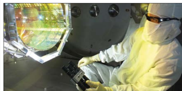
One of LIGO's mirrors is inspected by a technician.
