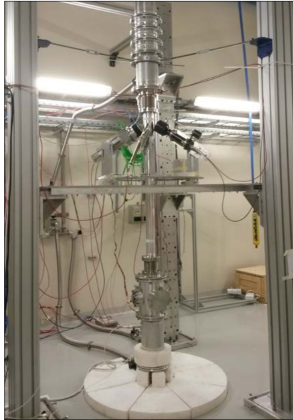
Fig. 3. The horizontal neutron beamline in EAR1 (left) and the vertical neutron beamline in the newly constructed EAR2.
