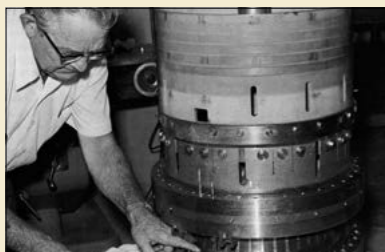
The body of the Stanford RCBC receiving the final touches before installation. It was successfully tested for two-million pulses at a rate of 20 Hz before data-taking started. The peak operating frequency of the chamber is 60 Hz.
