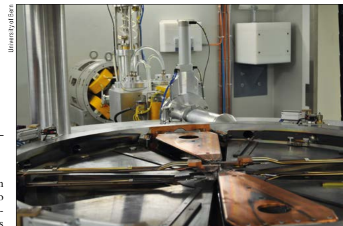
The acceleration chamber of the PET cyclotron, showing the out-port connected to the research beam transfer line.
