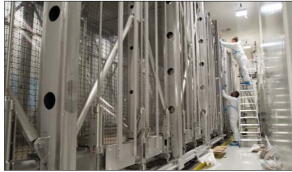
One of two 270m 3 modules for the ICARUS detector being refurbished by CERN and INFN, which will soon be filled with liquid argon to track neutrinos produced at Fermilab's short-baseline neutrino programme.
