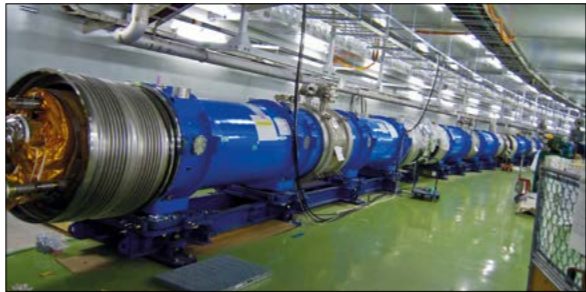
(Left) Hyper-K could be constructed from two huge cylindrical tanks each measuring 74 m in diameter and 60 m deep, containing a total of 600 thousand tonnes of highly purified water. (Right) Superconducting magnets at the Japan Proton Accelerator Research Complex (J-PARC) in Tokai village, which bend a 50 GeV proton beam towards the neutrino target. Plans are afoot to excavate Hyper-K a few kilometres from Super-K, so that it receives the existing neutrino beam from J-PARC, which will be upgraded to a higher intensity.
