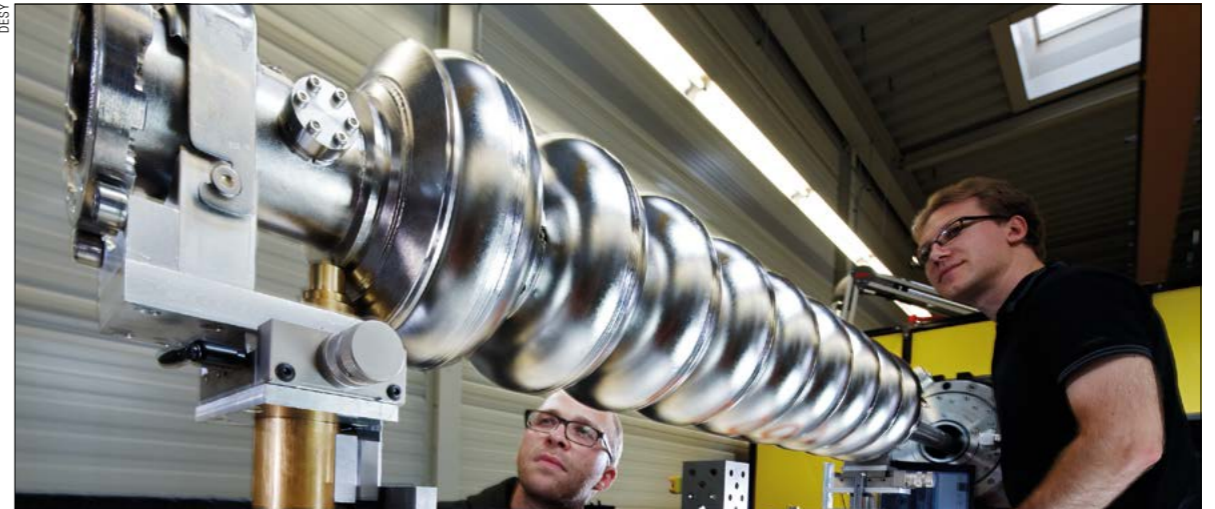
The ILC will need 16,000 of these superconducting radiofrequency cavities.
