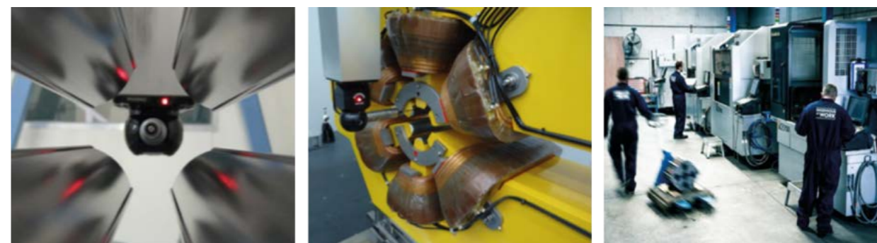
From left: CNC machined quadrupole pole inspection; EDM wire cut sextupole assembly; EDM wire cutting facilities at Buckley Systems.
