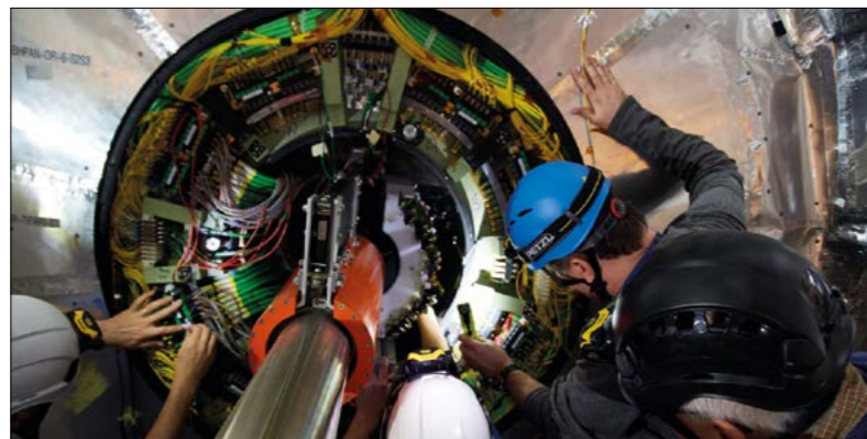
(Above and below) The new silicon pixel tracker being installed in the central region of the CMS detector.
