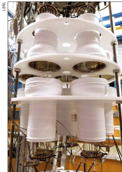
Photomultiplier tubes surrounded by polytetrafluoroethylene for the LZ experiment, which is managed by Lawrence Berkeley National Laboratory.
