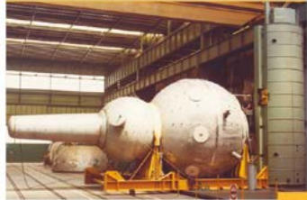
Vessel for the Sodium Pumps containment
