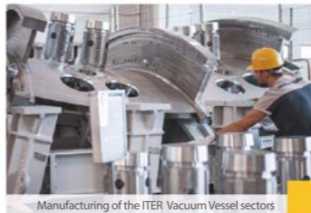
Manufacturing of the ITER Vacuum Vessel sectors
