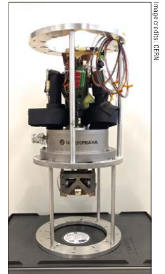
(Left) CT-PPS detectors installed in the LHC tunnel (CMS lies 200 m to the right). (Middle) Roman Pot upgraded with special RF shields for operation at high-luminosity. (Right) The new CT-PPS tracking detector package using 3D pixels to be used in 2017. The box at the bottom, containing six planes of silicon pixels, is inserted in the RP and the RP is mounted in a mechanical structure in the beamline that can be moved towards the beam.
