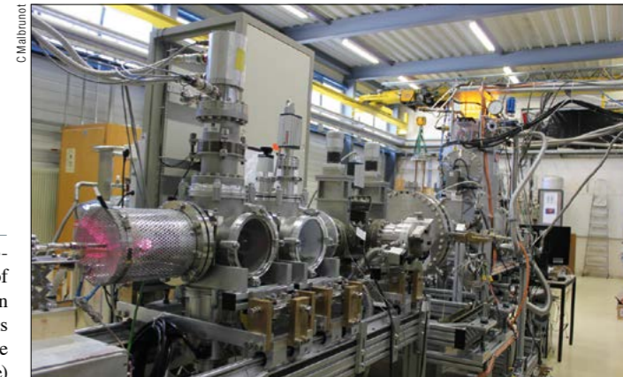
The ASACUSA experimental set-up, with the source of hydrogen visible by its characteristic pink glow.
