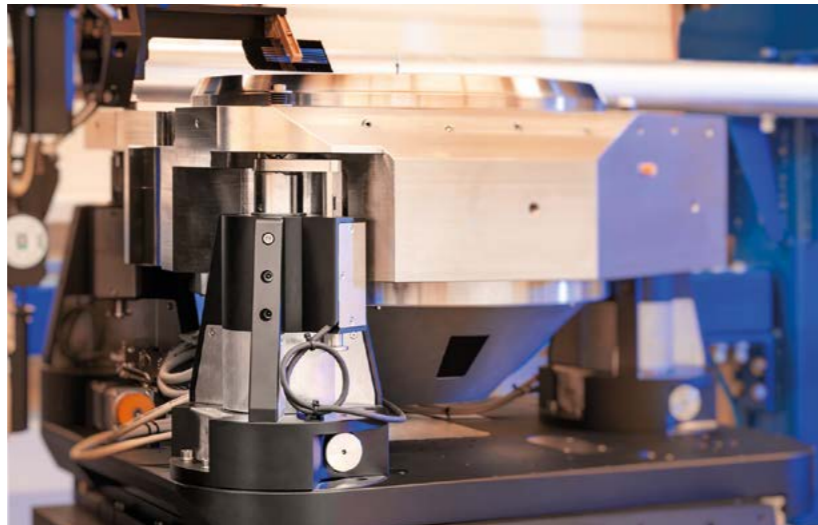
The Z lifting stage performs the height adjustment, tilt correction, and orthogonal alignment, relative to the beam (image: PI / HZG)
