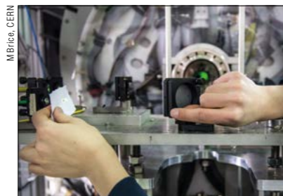
ALPHA uses a laser system to interrogate the electronic states of antihydrogen.
