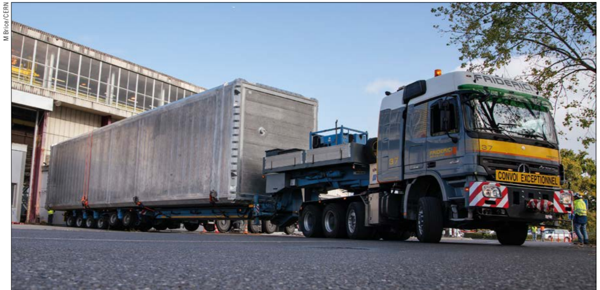
The cryostat for the ICARUS detector, one of three detectors that will make up Fermilab's short-baseline neutrino programme, being moved between buildings at CERN in late 2016 as part of its refurbishment programme, before being shipped to the US this summer.
