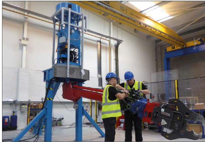
Prototype robotic arm developed as part of the remote handling solution for nuclear waste retrieval from the Dounreay Shaft
