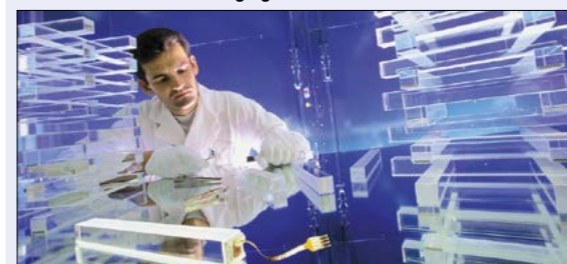
Dense, precision-grown crystals for the CMS experiment.
