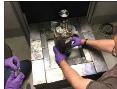
Placing the caesium-iodide detector, possibly the first handheld neutrino detector, in the path of the SNS beam.
