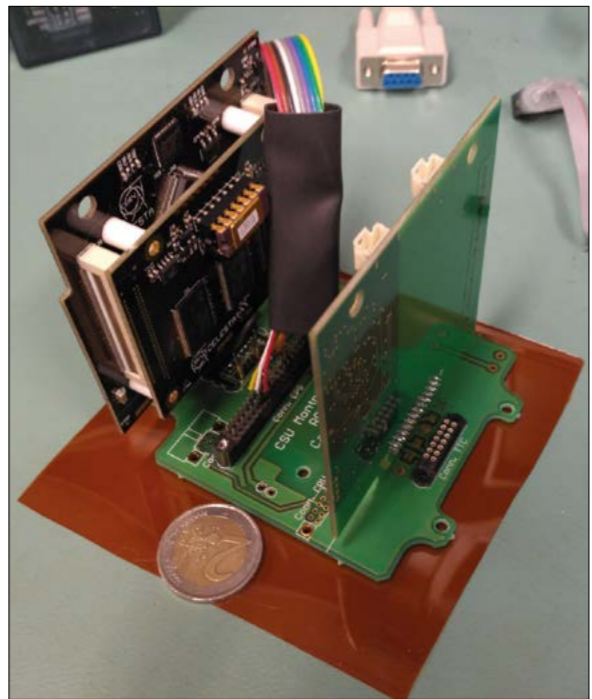
The CELESTA CubeSat payload module ready for radiation testing in CERN's CHARM facility.
