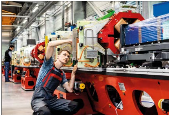
Inspecting a girder carrying elements of a single EBS cell.
