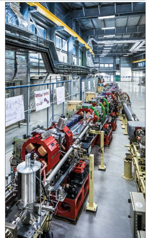
A mock-up of the new storage ring with an X-ray beamline branching off to the right.
