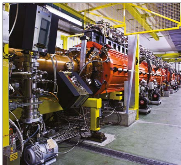
Fig. 2. The Linac2 RFQ pre-injector and duoplasmatron proton source attached to the machine's RF tanks, photographed in 2008.
