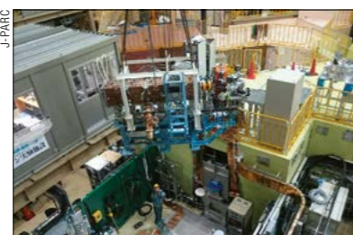
(Left) Installation of the RFQ in the experimental area. (Right) When turning on the RFQ (red), a peak is observed at the expected timing (green). The peak disappears when turning off the RFQ (blue), suggesting acceleration has taken place.
