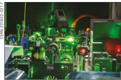
ISOLDE's resonant ionisation laser-ion source (RILIS), which provided the first beams of neutron-rich chromium isotopes.
