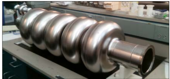
Fig. 4. The 802 MHz five-cell RF cavity, produced in a partnership between JLAB and CERN, has achieved accelerating fields exceeding the FCC requirements.
