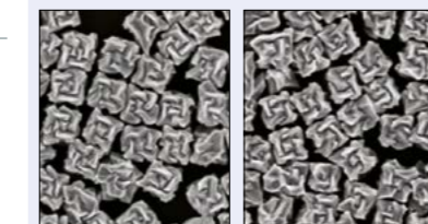
Scanning electron microscope images of chiral gold nanoparticles grown in the presence of L (left) or D (right) amino acids.
