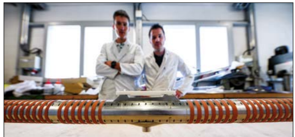
Fig. 5. First beam screens for a high-energy FCC proton–proton collider. Based on a novel vacuum system with improved heat transfer, lower impedance, improved pumping and feasible manufacturing, the design mitigates the formation of electron clouds and removes the much higher synchrotron-radiation power.
