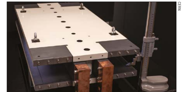
Fig. 2. Left: winding of the enhanced racetrack model coil (RMC) for FCC-hh 16 T magnets with Nb 3 Sn superconducting cable at CERN. Right: A 1 m-long prototype of the FCC-ee dipole magnet. The proposed design considerably reduces the power consumption and the total amount of material required. For example, a machine three times longer than LEP will only require around 35% more steel.
