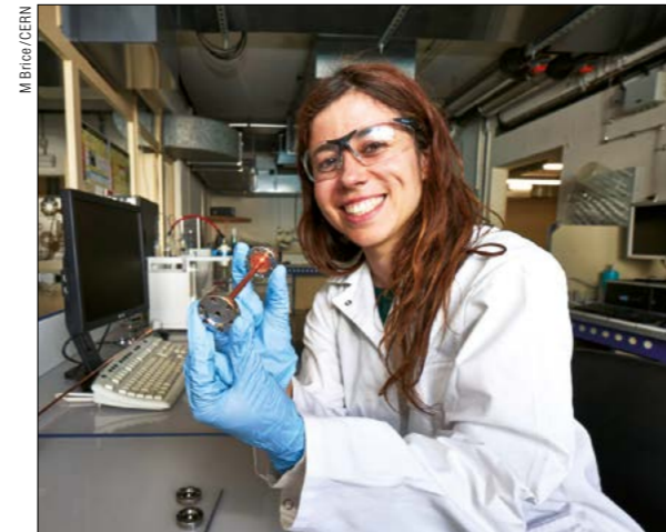
Fig. 3. Prototype of a NEG-coated vacuum chamber produced by copper electroforming and coated using a sacrificial mandrel. The technique is applicable to a wide range of diameters and lengths.
