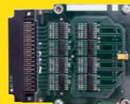
A395A - 32 LVDS/ECL/PECL input channels
