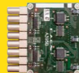
A395D - 8 NIM/TTL input/output channels
