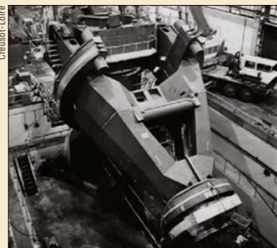
The top part of the telescope structure. In the foreground is the main body of the polar axle and the U-shaped journal bearing fitted with its two counter-weights.
