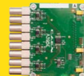
A395E - 8 Analog output 16-bit channels
