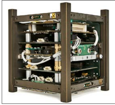
CELESTA contains a space version of CERN's radiation-monitoring system RadMon, and is the first full satellite tested in the CHARM facility.
