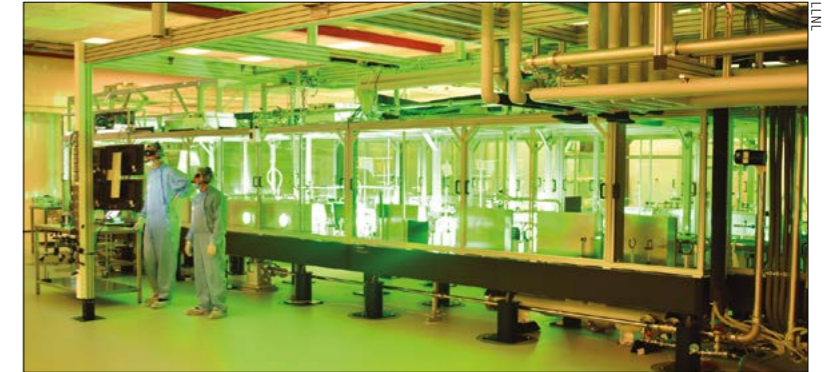
Chirped-pulse amplification gives extreme lasers sufficient peak power to accelerate electrons up to multi-GeV beams, such as the High-Repetition-Rate Advanced Petawatt Laser System (HAPLS) recently installed at the Extreme Light Infrastructure facility in the Czech Republic.
