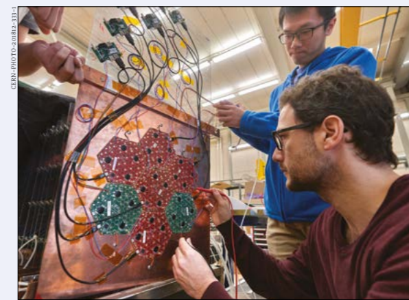
Prototype sensors The assembly of prototype HGCal detector planes, based on 6" silicon modules, at CERN in October.
