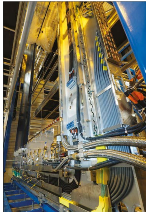
Development The SciFi tracker modules being assembled.
