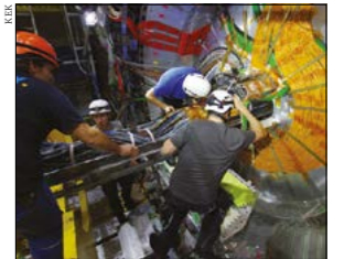
The vertex detector being incorporated into Belle II.
