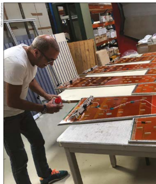
Assembly The production of the GEM chambers to be installed in the muon endcaps during LS2.
