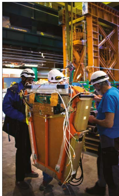
Endcap petals Assembling cathode strip chambers during the end-of-year-shutdown in 2017/2018.
