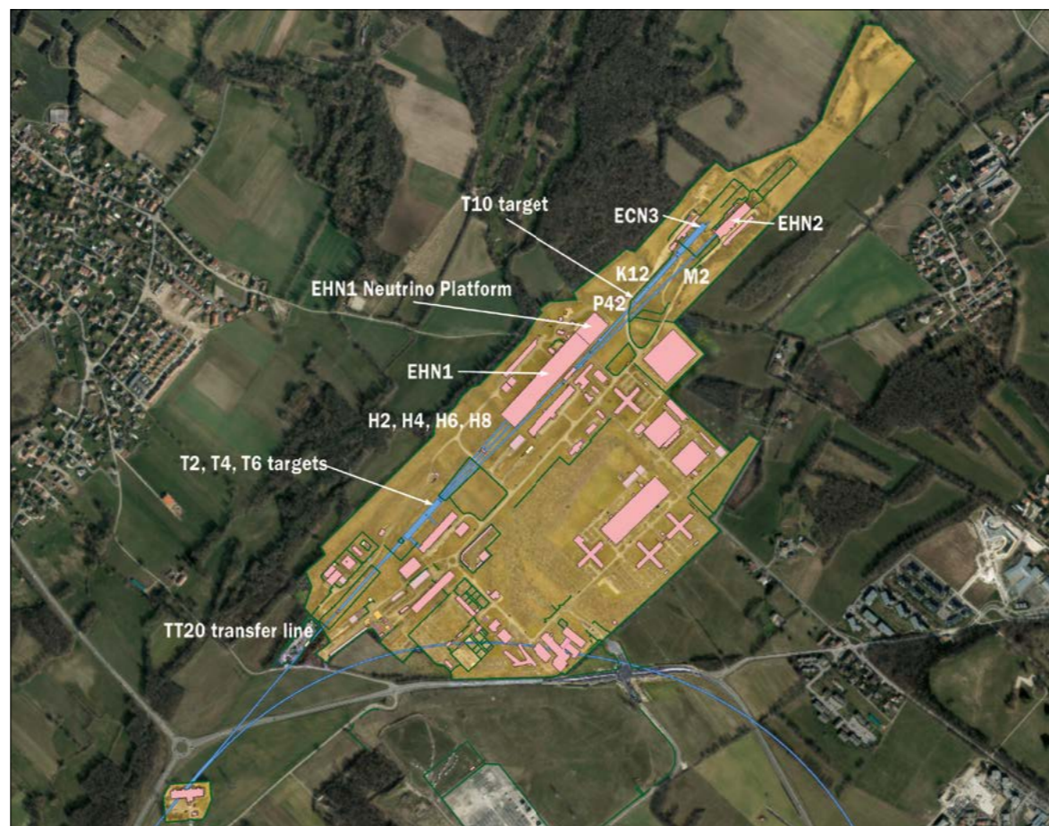
North Area Protons leaving the SPS enter a target station (bottom left), leading to 6 km of secondary beamlines for experiments in three halls.
