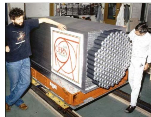
Spaghetti calorimeter Riccardo de Salvo (left) and Alois Sigrüst at CERN in 1990 with a lead-fibre prototype that held the record for energy resolution of single hadrons for 25 years.
