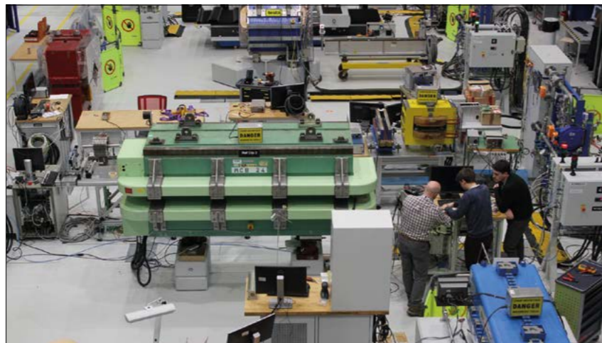
2D sense Paragraf and CERN scientists setting up the graphene Hall sensor for performance evaluation in the reference dipole magnet of CERN's magnetic measurement section.
