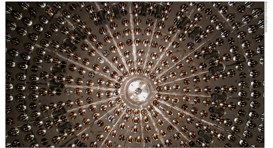
Solar focus Borexino's 2200 photomultipliers detect scintillation light generated by electron/positron recoils induced by sub-MeV neutrinos.
