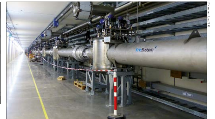
Cool view A section of the cryogenic system for the 600 m-long linear accelerator.
