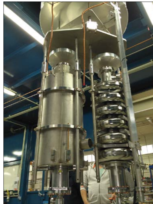
Vertical test The first cavity of the ESS elliptical section developed by INFN, seen here on the left (next to a large-grain prototype), being prepared for a vertical test at DESY before shipment to CEA Saclay for assembly in the cryomodule.
