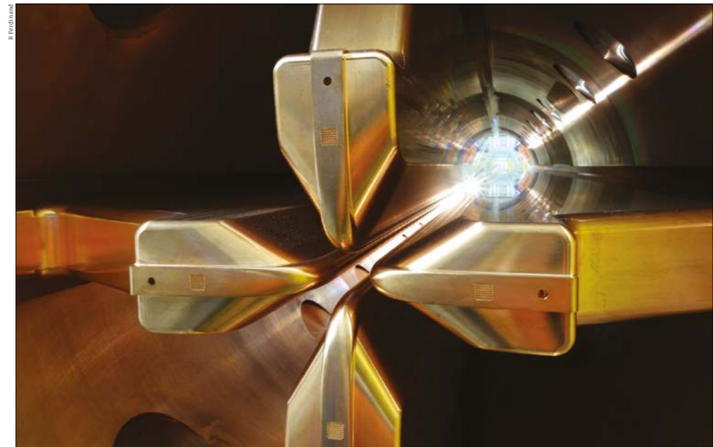
On the plus side Inside view of the radio-frequency quadrupole at the entrance to SPIRAL2's superconducting linear accelerator.
