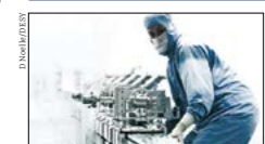
On the cover: Roll-out from a DESY cleanroom of a 3.9 GHz RF cavity string for the European XFEL. 35
