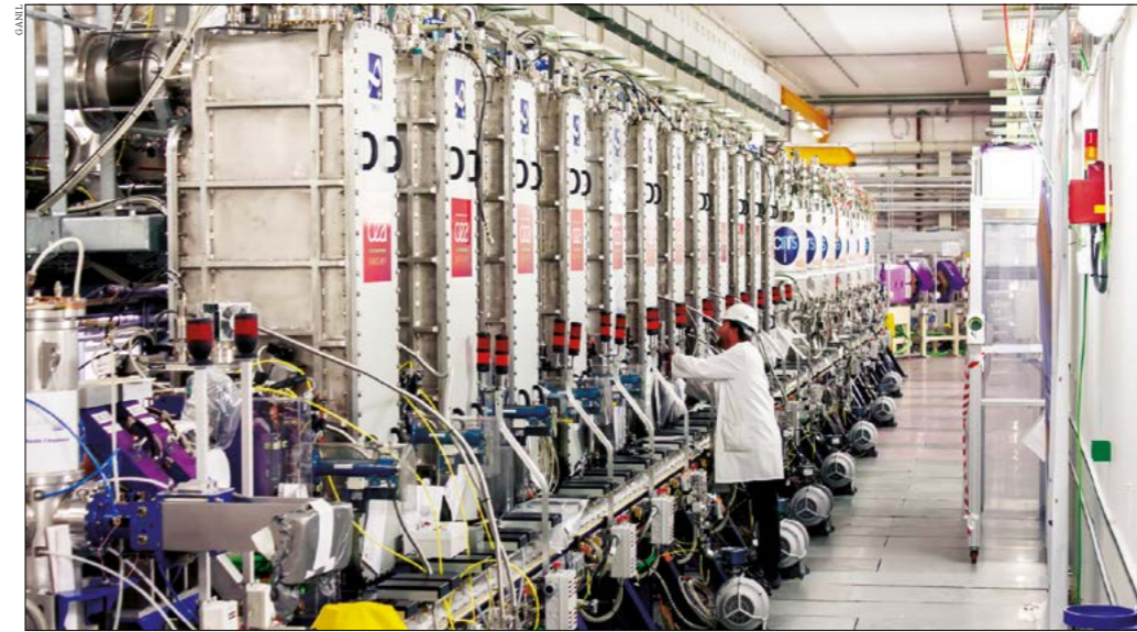
Multitasking The nineteen superconducting cryomodules of the SPIRAL2 linac.
