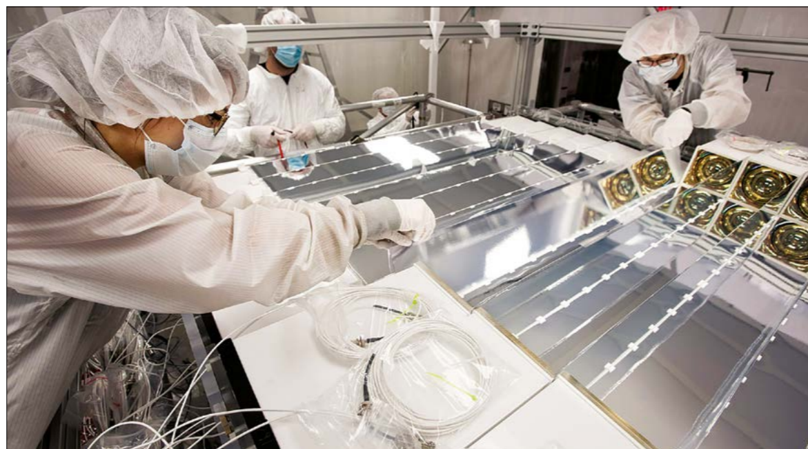
Technology demonstration Technicians assemble the PROSPECT neutrino detector, which was installed a few metres from the High Flux Isotope Reactor at Oak Ridge National Laboratory in Tennessee. Similar technologies could be used to monitor nuclear reactors.
