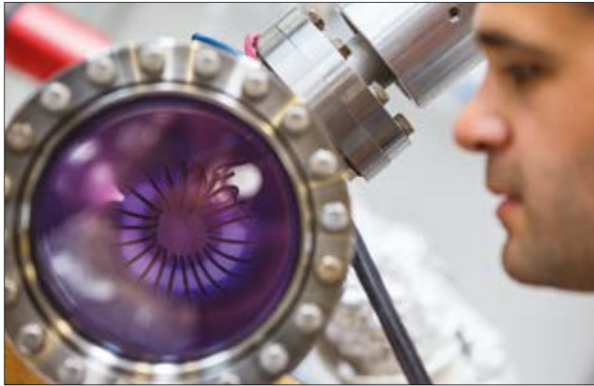
Magneto-sputtering A researcher experiments with a technique for applying a thin superconducting film to radio-frequency (RF) cavities. Superconducting RF is a key technology for the sustainable operation of the FCC as a Higgs and electroweak factory.
