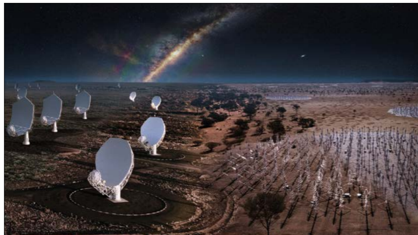
Split screen The two future SKA telescope arrays, in South Africa (left) and Australia (right), will deliver approximately 8 Tb/s to two supercomputers, before distributing and storing up to 700 PB of data each year.
