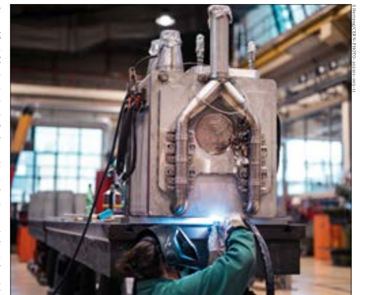
Neutron production target Welding of the upstream cover and proton window on n_TOF’s third generation lead-based neutron spallation target.
