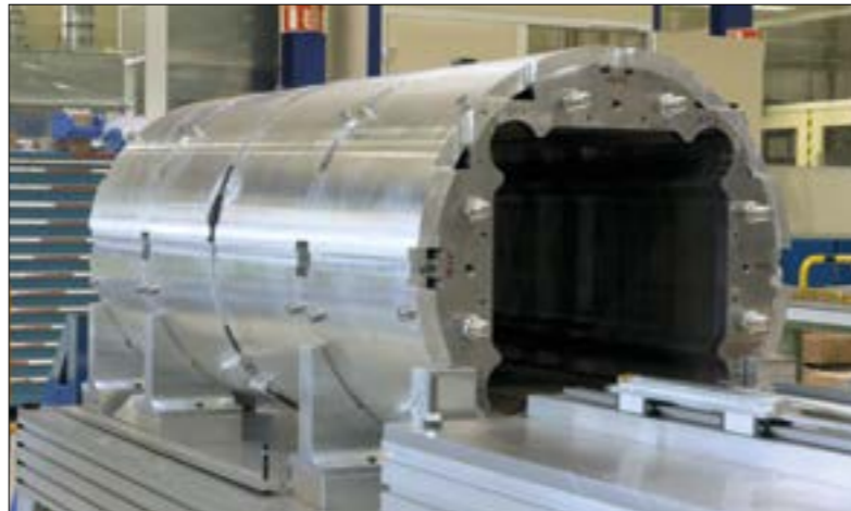
An example of an MQXF magnet. ARMCO® Pure Iron is specified for LARP low-beta quadrupole master keys, yokes and load pads.
