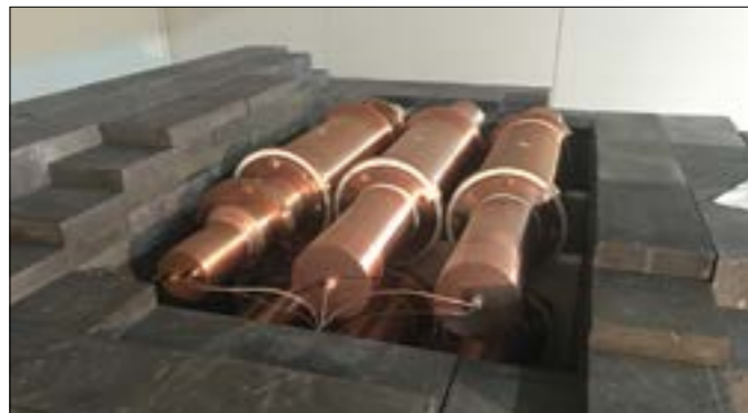
Still in the dark Photomultiplier tubes for ANAIS inside their shielding blocks and (right) a comparison between the ANAIS and DAMA/LIBRA results.
