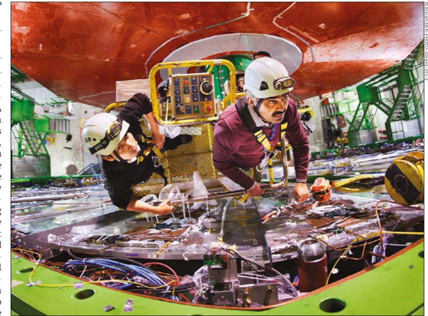
Muon detector Resistive-plate chambers in the CMS detector (grey disk), pictured during the ongoing second long shutdown of the LHC.
