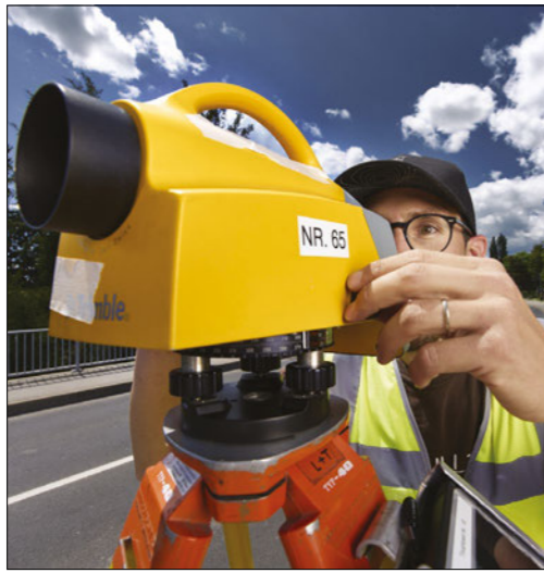
Level headed CERN's Pierre Valentin performing levelling measurements between Certoux and Saint-Julien in France.
