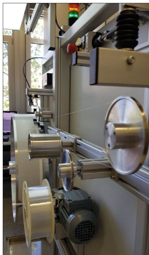
SciFi spools Scintillating-fibre mat production at EPFL, Lausanne, in 2017.
