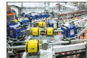
The S-DALINAC linac has been operated in energy-recovery mode.
