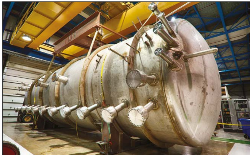
Trailblazing TPC MicroBooNE can shed light on the MiniBooNE anomaly by differentiating electromagnetic showers from electrons and photons.
