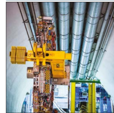
Descent into the pit The ATLAS experiment's New Small Wheels are now being installed. 27
