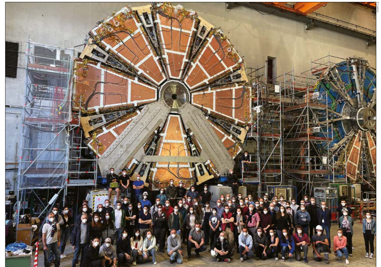
Revolutions The first of the ATLAS New Small Wheels (NSW-A) ready for transport to Point 1 of the LHC. On the right is NSW-C where, at the time of the photograph in July 2021, only a few sectors had been installed.
