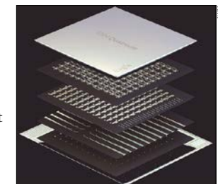
IBM’s multi-layer “Eagle” processor.
