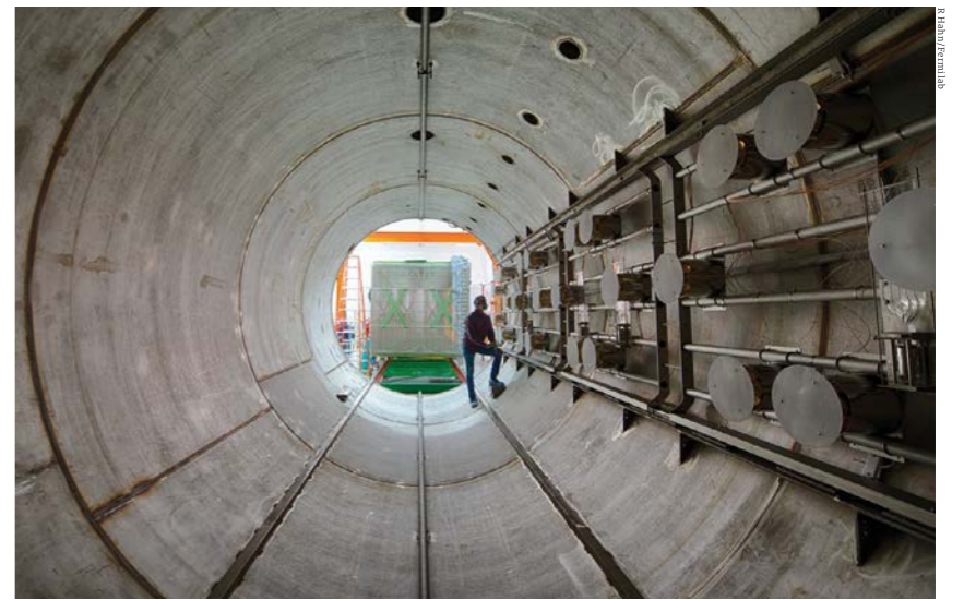
Cross check The MicroBooNE experiment’s liquid-argon time-projection chamber is inserted into its cryostat.
