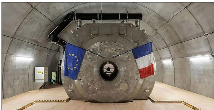
Flying the flag The front face of the high-field niobium-titanium MRI magnet.
