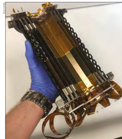
Pioneering pixels Left: half of the SLD vertex detector, consisting of 307 Mpixels, three barrels and a pixel size of 20 \times 20 \times 20 \mu\text{m}^3 . Each ladder of 16 cm active length contains two 8 cm-long stitched CCDs. Top right: CGI of the original ATLAS pixel detector, comprising 92 Mpixels ( 50 \times 400 \mu\text{m}^2 for the external layers and 50 \times 250 \mu\text{m}^2 for the innermost layer). Bottom right: simulated tracks in the MAPS-based ALICE ITS2, containing 12.5 Gpixels and a 10 \text{ m}^2 active area (see p29). To offer a sense of scale, the entire SLD vertex detector would fit within the innermost layer of the ATLAS pixel detector.
