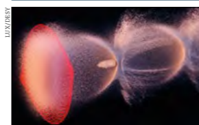
An electron bunch (centre) surfs on a plasma wave of electrons (white) driven by a laser pulse (red).
