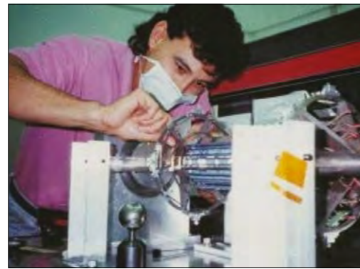
Top detector Bert Gonzalez with the SVX microstrip vertex detector of the CDF experiment at the Tevatron in 1993, which was instrumental in the co-discovery of the top quark.
