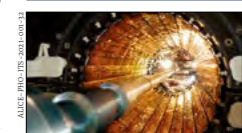
On the cover: The outer barrel of ALICE's new inner tracking system installed in March. 29
