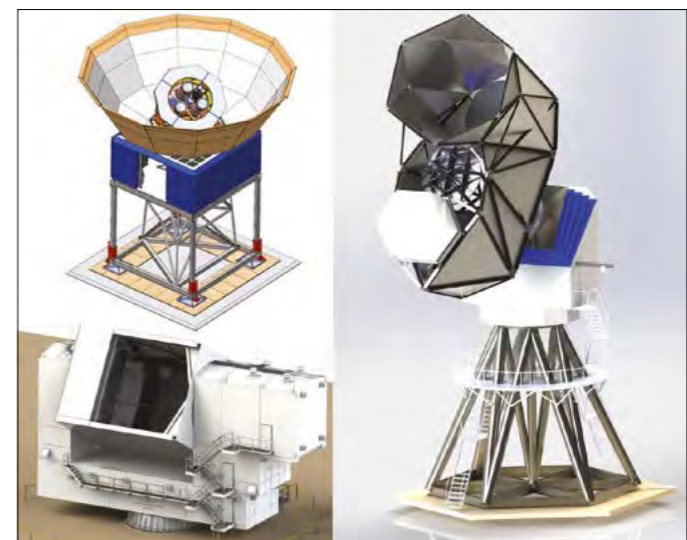
Looking up The full facility will employ 18 0.5 m small-aperture telescopes (top left), three per mount, fielding 150,000 detectors; one 5 m large-aperture telescope (right) fielding 130,000 detectors; and two 6 m large-aperture telescopes fielding 275,000 detectors (bottom left).
