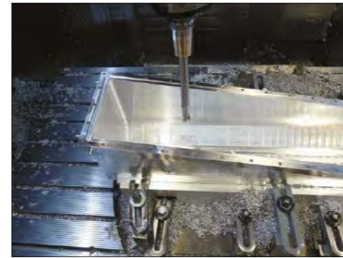
RF boxes Milling the solid aluminium block (left), and the completed RF foils in the closed position (right).
