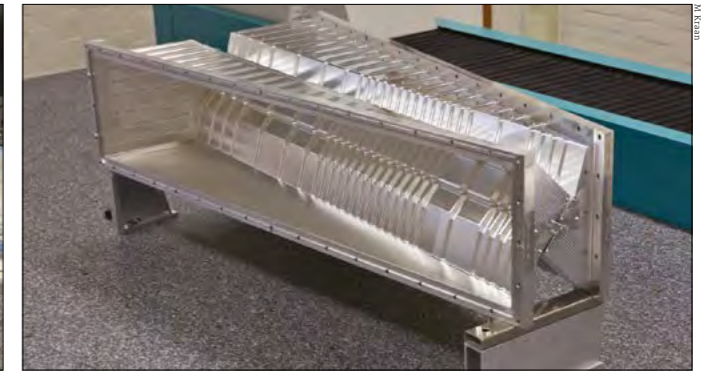
RF boxes Milling the solid aluminium block (left), and the completed RF foils in the closed position (right).
