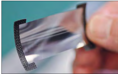
IDEAs Curved silicon with a 2.5 cm radius of curvature on a carbon-fibre support, demonstrating the feasibility of making low-mass, rigid FCC-ee detector systems.
