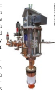
RF boost The first commercial prototype of a high-efficiency 8 MW, 12 GHz "E37117" klystron.
