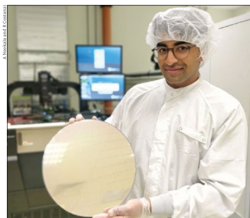
Outer tracker Top: an outer tracker barrel ladder with modules equipped with strips running up to the middle of the sensors and read-out at both ends. Left: a 12-inch 65 nm-technology wafer used as the basis of the read-out of the outer tracker, which joins a total of 25 m 2 of ASICs and sensors by bump-bonding. Right: a final mechanical ring design depicting the concept of tilting modules towards the interaction point, with thermal performance (inset) verified to be excellent.
