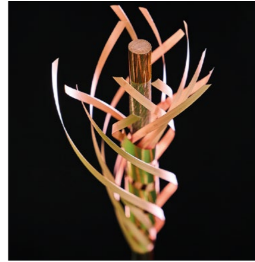
Hot stuff CERN's superconducting rare-earth barium copper oxide (also referred to as REBCO) power-transmission cable, used to study the feasibility of high-temperature superconductivity for aircraft.
