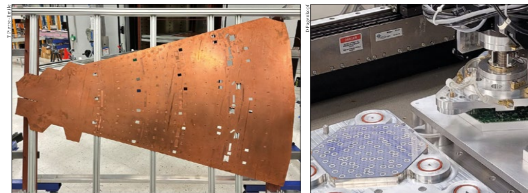
High-granularity calorimetry Left: a cooling plate in the hadronic section, providing the base for the hexagonal silicon modules (to left of plate) and the rectangular SiPM-on-tiles (right). Right: automated high-granularity calorimeter silicon-module assembly, showing the gantry joining the hexagonal 8-inch pad sensor with glue circles to the read-out board electronics.
