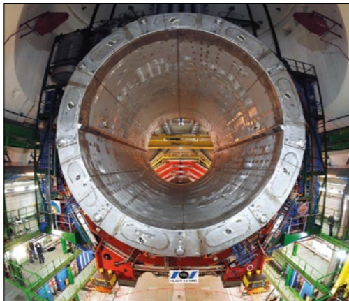
One of a kind The large Nb-Ti superconducting magnet of the CMS detector being installed in 2007.
