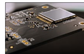
The multipurpose hybrid pixel detector chip Timepix3.
