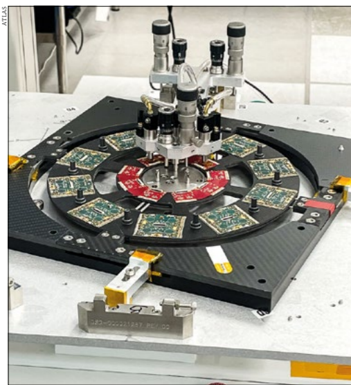
ITk prototyping Loaded prototypes for (left) a pixel end-cap ring of the inner system and (right) a strip barrel stave of the ITk detector.
