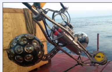
Stepping stone A prototype of the KM3NeT DOM was tested on an ANTARES line in 2013 and recovered in June 2022.
