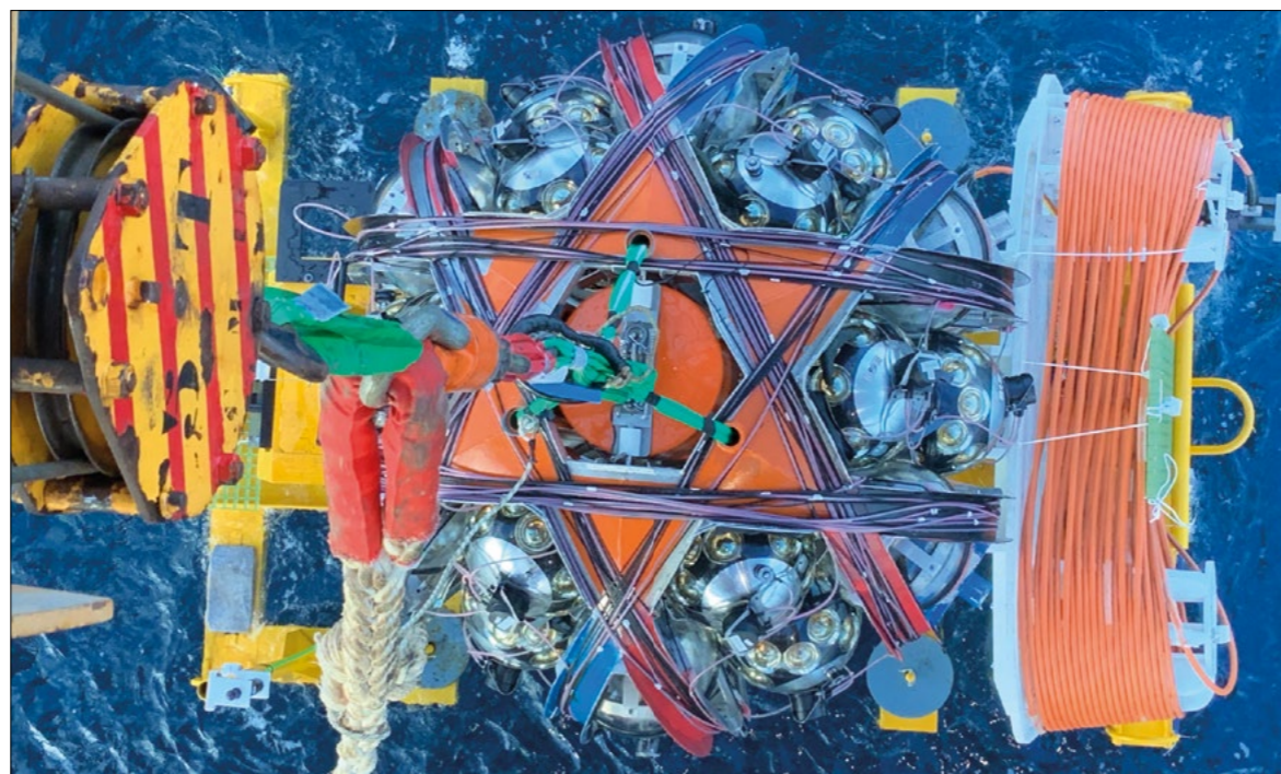
First descent One of the KM3NeT lines bundled up before being unwound and lowered into position.
