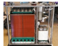
High Voltage Pulse Transformer & Pulse Modulator
