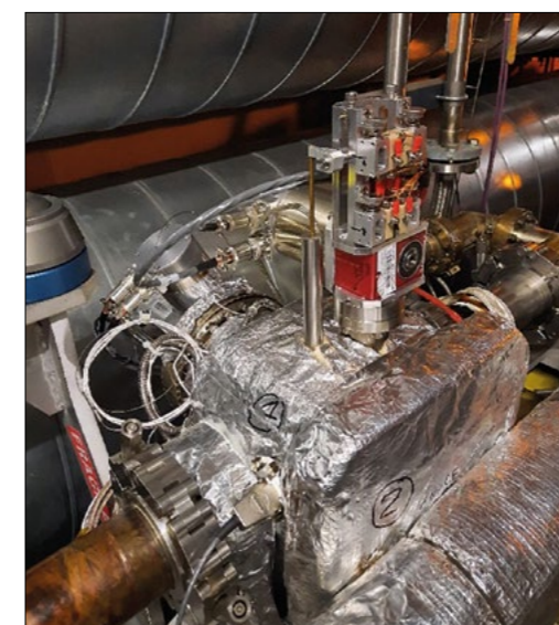
Silicon swerve Top: a silicon-strip crystal (built by INFN Ferrara) used for LHC beam collimation, which is bent to an 80 m-curvature radius to produce a 50 \mu\text{rad} kick. Bottom: the vacuum tank in the LHC housing the bent crystal and interferometer head used during beam tests to control the crystal’s orientation.
