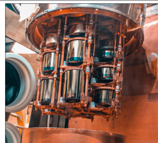
High resolution Germanium cells in the Majorana Demonstrator cryostat, some of which were exchanged with tantalum to search for dark matter in the decay of metastable tantalum-180.
