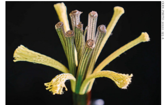
Flourishing A magnesium diboride cable, 19 of which are twisted together inside a compact, flexible cryostat to provide one of eight superconducting links powering the HL-LHC magnets.
