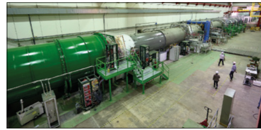
Intense Part of the NA62 detector in the ECN3 experimental hall in Preveessin, where beam travels from right to left. On the right-hand side is the STRAW spectrometer, with the analysing magnet in blue. Four large-angle vetoes serving to clean the samples from non-forward events are visible in white, while the green region houses the RICH detector.
