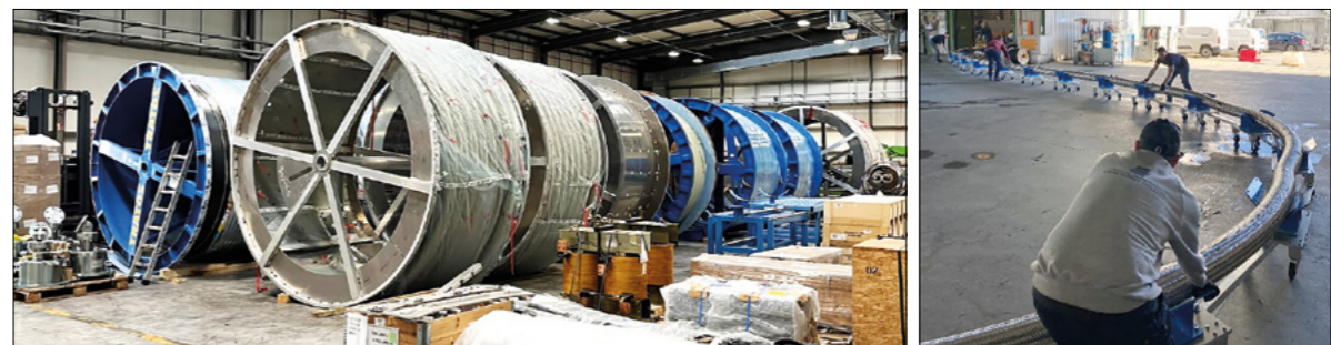
kA currents Delivery and handling of the 120 kA MgB 2 cable assembly. The flexible, double-walled corrugated cryostat comprises 19 MgB 2 superconducting cables in a single assembly, twisted together to form a compact bundle. Each MgB 2 cable is about 140 m long with the bundle diameter around 90 mm.
