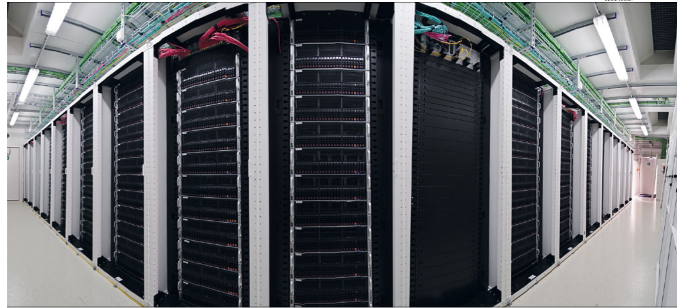
New nodes The event processing node racks in the ALICE computing farm, part of a completely new computing model for Run 3 and beyond.
