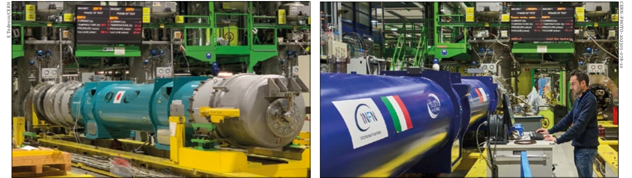
Dipole magnets Prototypes of a single-aperture dipole D1 (left) and a twin-aperture dipole D2 (right) on the test bench in SM18.
