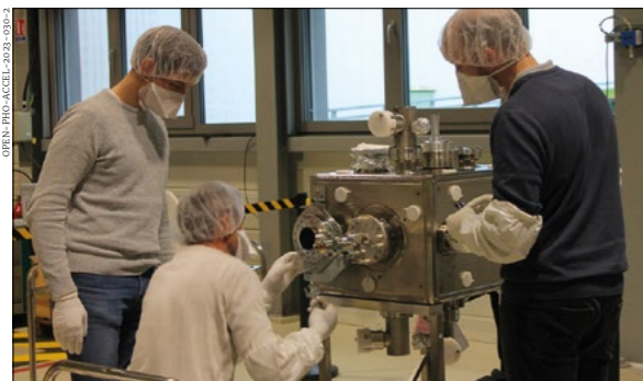
Crab cavities The insertion of a beam screen in a DQW crab cavity (left) and the arrival and unpacking of the RFD cryomodule (right), both in the SM18 hall in November 2023.
