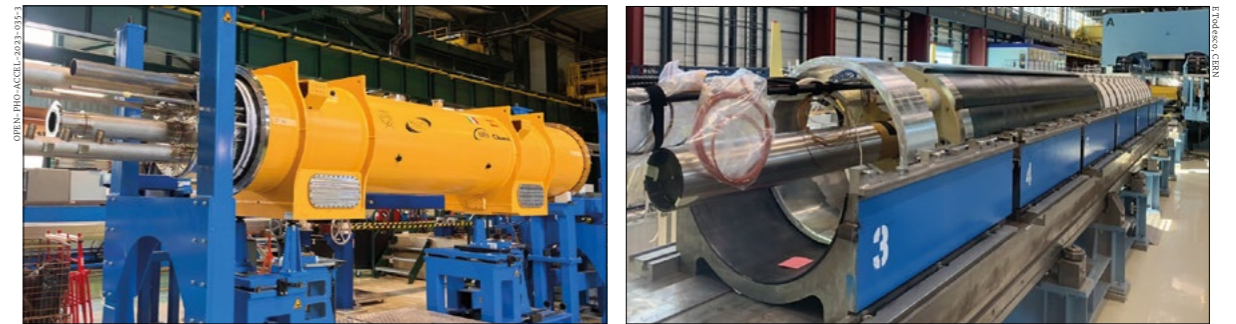
Corrector magnets An HL-LHC corrector package in its cryostat (left) and construction of the corrector-magnet cold mass (right).
