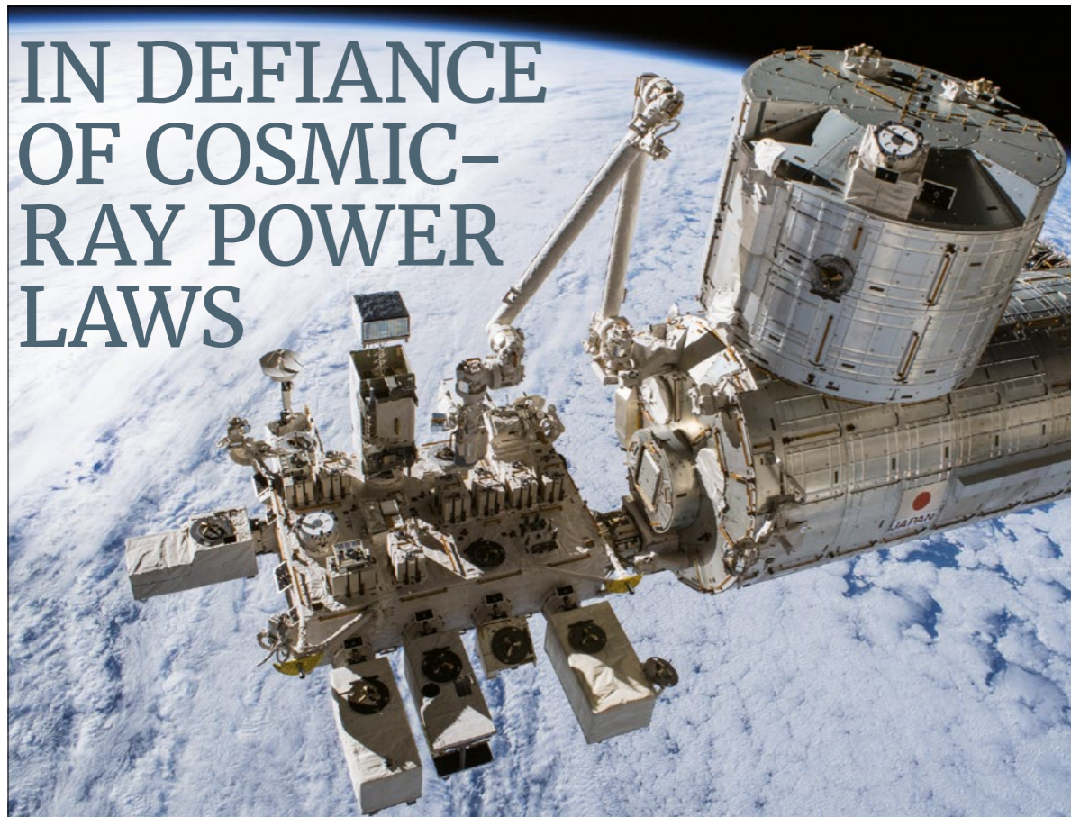
Low-Earth orbit The Calorimetric Electron Telescope (extreme left), attached to the exposure facility of the Japanese Kibo module at the ISS.
