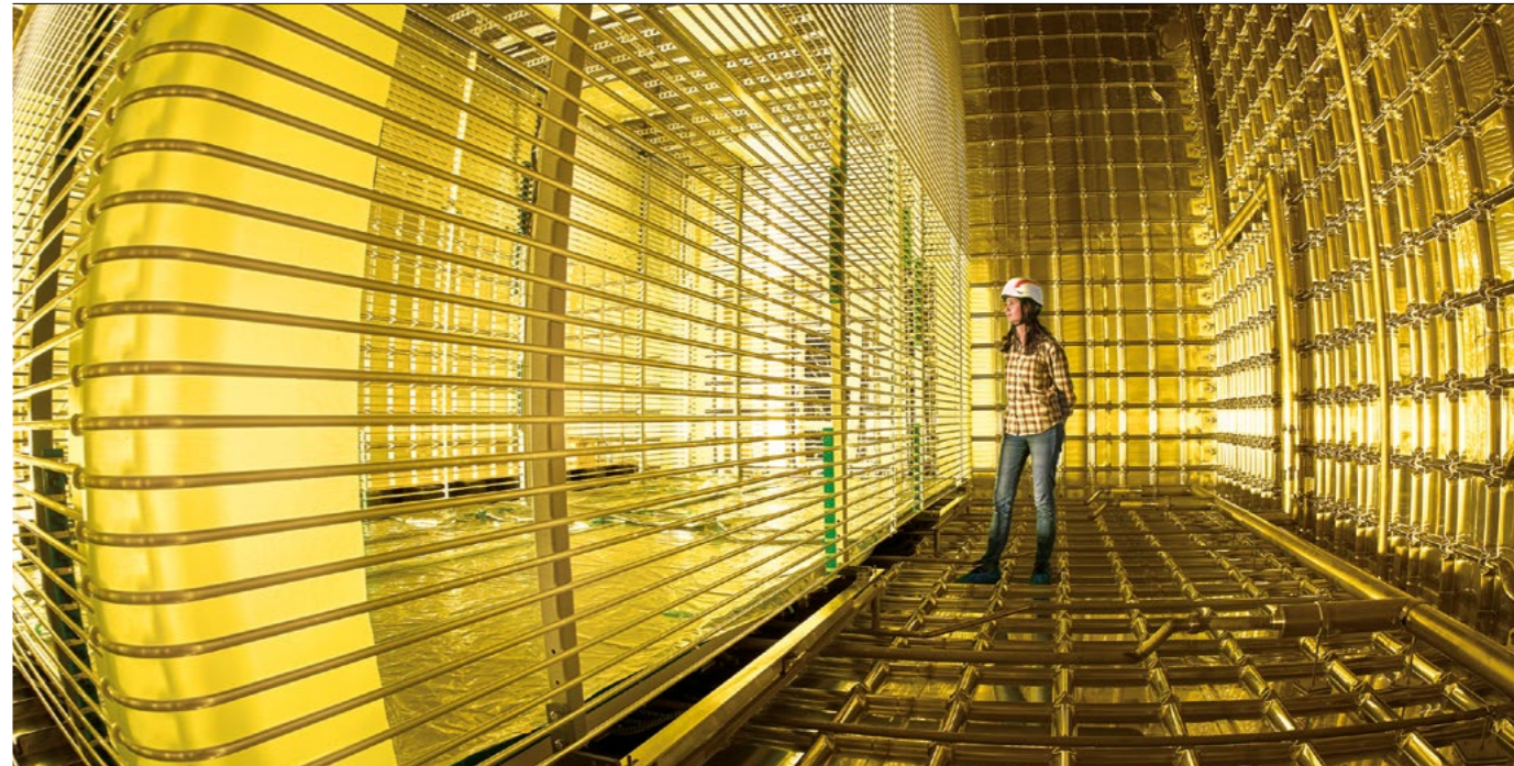
Vertical drift A physicist studies the field cage of a prototype liquid-argon time-projection chamber at CERN.
