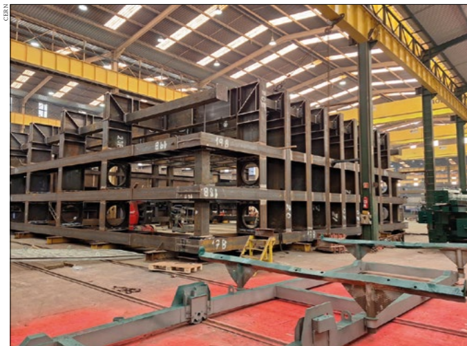
Cryostat creation The pre-assembly of a section of the second cryostat for DUNE at the factory in Arteixo, Spain.
