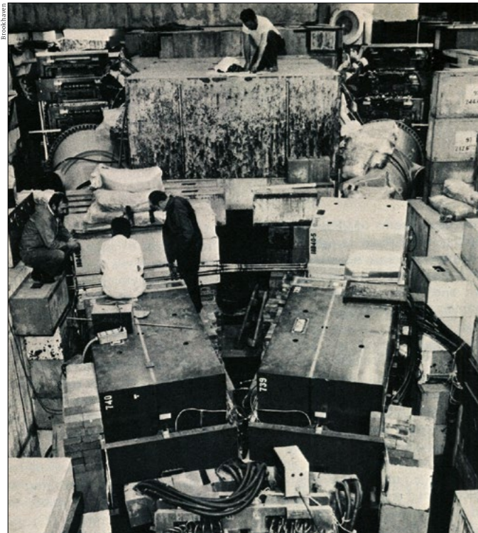
Fork in the path The detection system of the experiment at Brookhaven that spotted the new particle. It consists of two symmetrical spectrometer arms, 20 m long. In the foreground in each arm are three magnets. They are followed by Cherenkov counters (looking like cement mixers) to identify particles (in addition to Cherenkovs in the magnets) and, finally, multiwire proportional chambers which determine precise particle positions.
