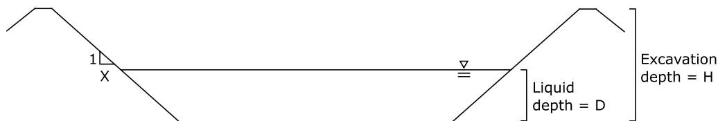
Figure 13. Profile view of typical manure storage lagoon construction. Not drawn to scale; the vertical scale on this diagram is exaggerated to show the side slopes and liquid level clearly.
