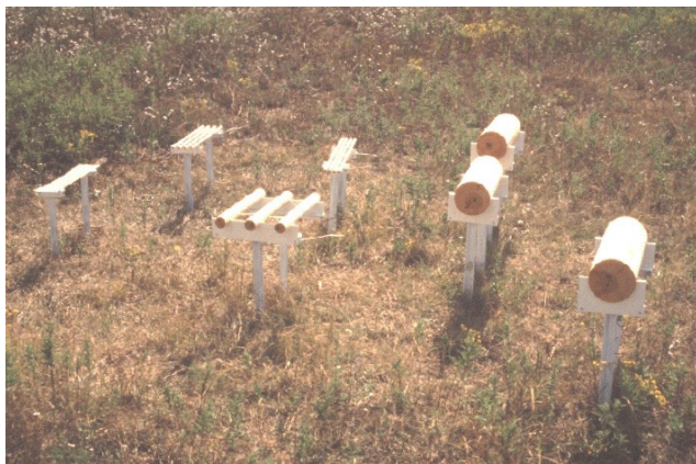
Fuel sticks in the field representing the four time-lag sizes. 1-hour dead fuels are on the extreme left (0.125" diameter); 10-hour are in the back left area (0.5" diameter); 100-hr are in the center front (1.5" diameter); and 1,000-hour are on the right (5" diameter).
