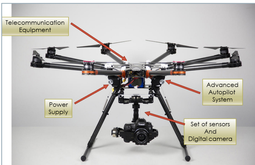
Figure 4 UAV equipped with the digital camera and set of sensors Source: Hristov, Zahariev and Beloiev
