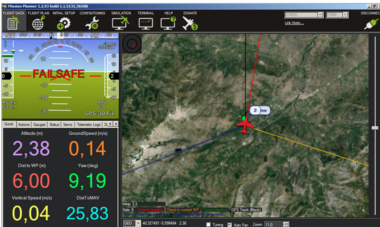
Figure 7 Graphical User Interface (GUI) software for mission planning (Mission Planner Software)
