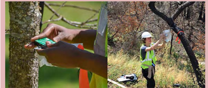
Figure 2: AudioMoth sound recorder (left) and device deployment in a burned area (right).
