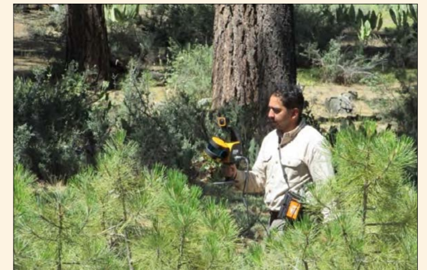
Figure 2: HMLS scanning of a plot.
