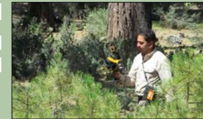
2 SONOMA & SAN LUIS OBISPO Using handheld LiDAR scans of Heterobasidion irregulare affected plots
