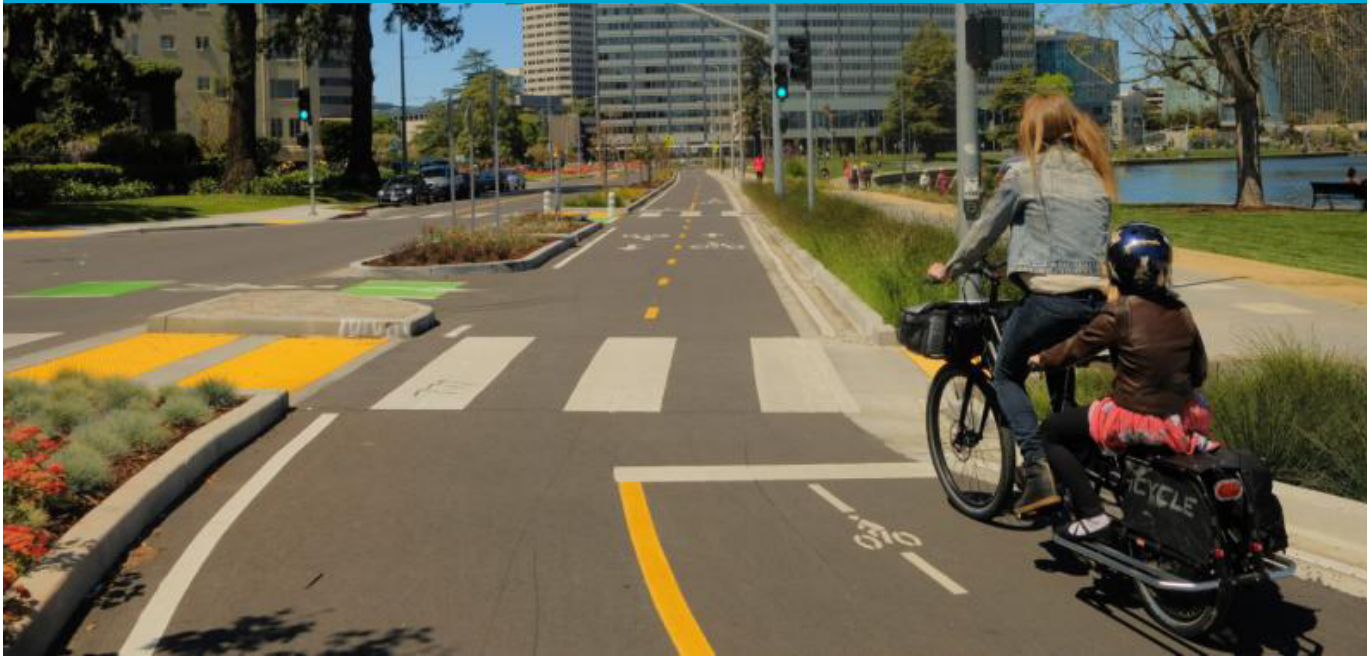
Riders using two-way cycletrack in Oakland, CA, USA. Source: Kyle Ramey of Bikabout
