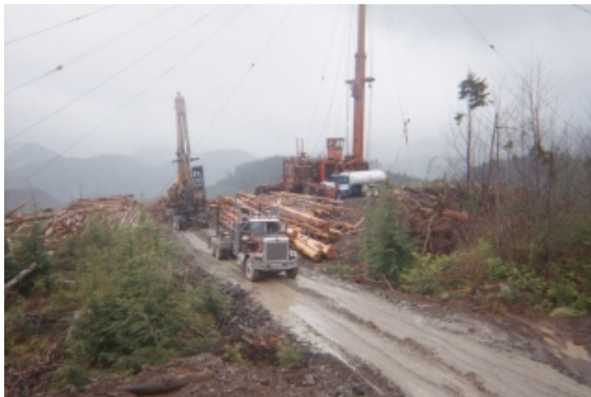
Figure 1: Berger Mark VI tower yarder operating in second-growth forests
