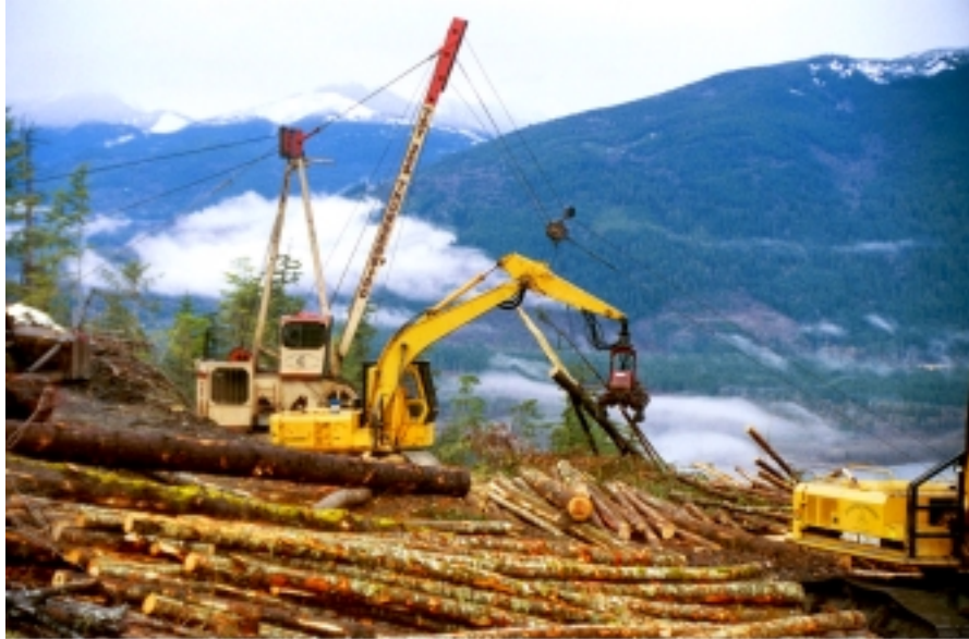
Figure 6: A redesigning the TB 255B SLR results in a versatile yarder. Shown here is an example of a TSY 255
