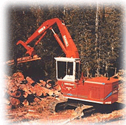
Figure 2: A 3800C log loader that can be used for shovel yarding
