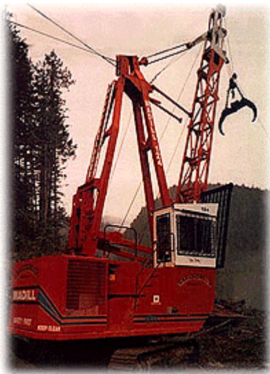
Figure 4: The Madill 124 Swing Yarder in grapple configuration
