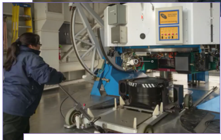
Karen Kinemuchi loads the cartridge containing the aluminum plate and fiber optic cables into the spectrograph that is attached to the back end of the
