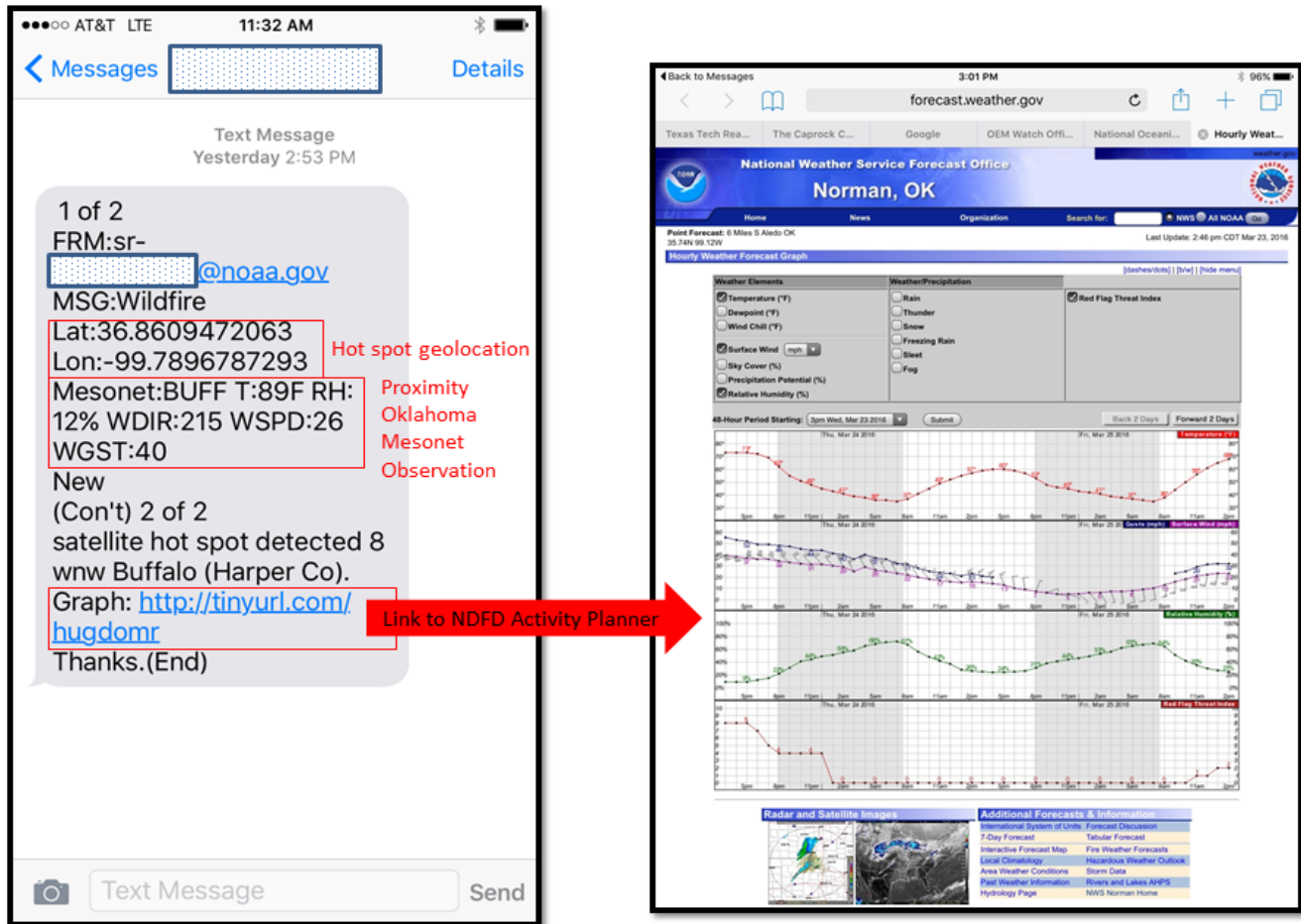
Figure 4. Example cellular text messaging output (left) of the wildfire notification with hot-spot geolocation, Oklahoma Mesonet proximity observation, and linked NDFD activity planner for selected fire weather parameters (right). Contact information is obscured.
